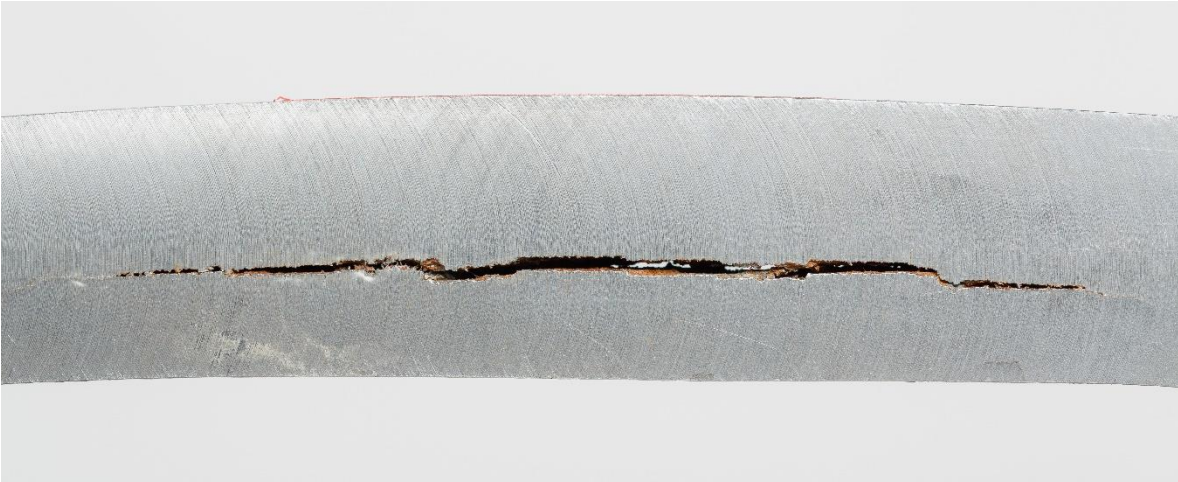
Damage Mechanism: Hydrogen Embrittlement, also known as Hydrogen Induced Cracking (HIC) © CEphoto, Uwe Aranas
