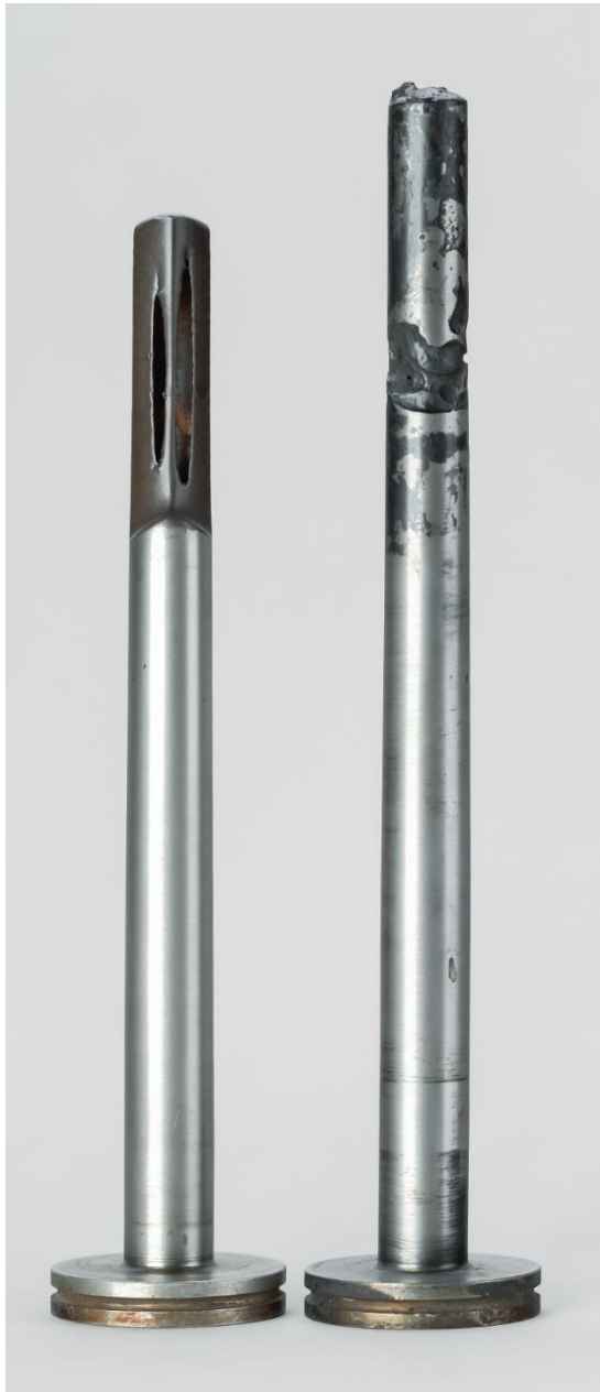
Different types of degradation of thermowells with considerable material loss due to erosion and corrosion attacks © CEphoto, Uwe Aranas
