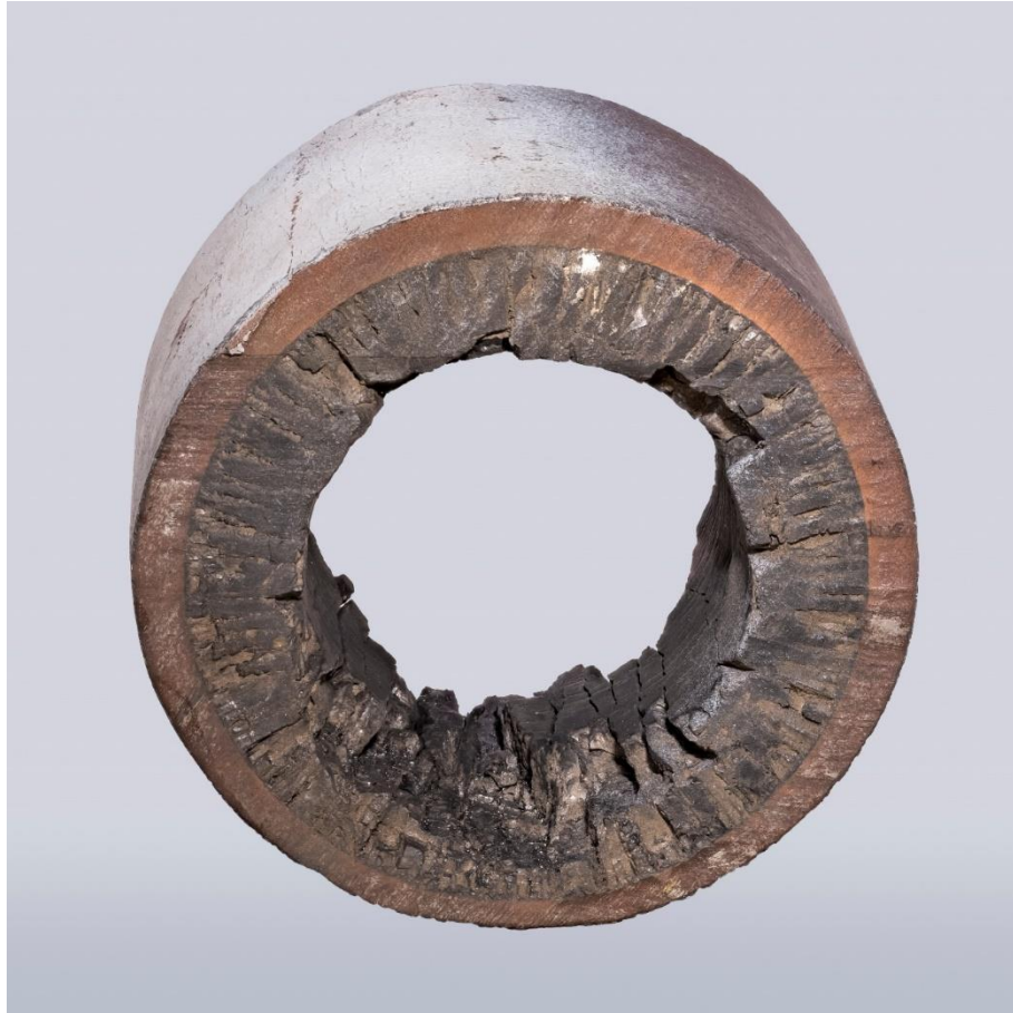
Scaling and Cracking of a 12CrMo19-5 tube © CEphoto, Uwe Aranas
