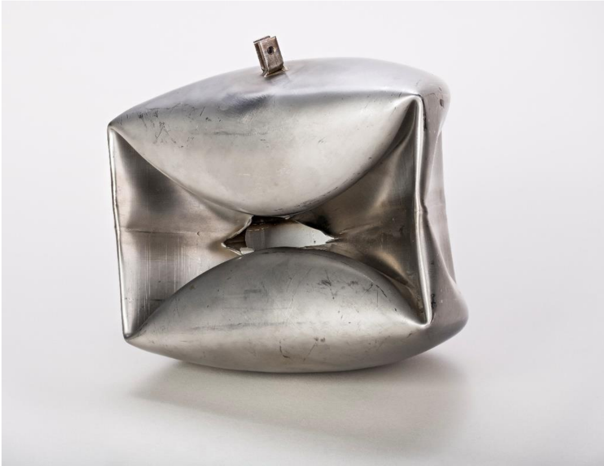
A float gauge of a separation vessel, destroyed by a Joukowski Pressure Shock from an interconnected fluid pipeline. The pressure shock squeezed the symmetric float gauge until it burst as consequence of the external overpressure © CEphoto, Uwe Aranas
