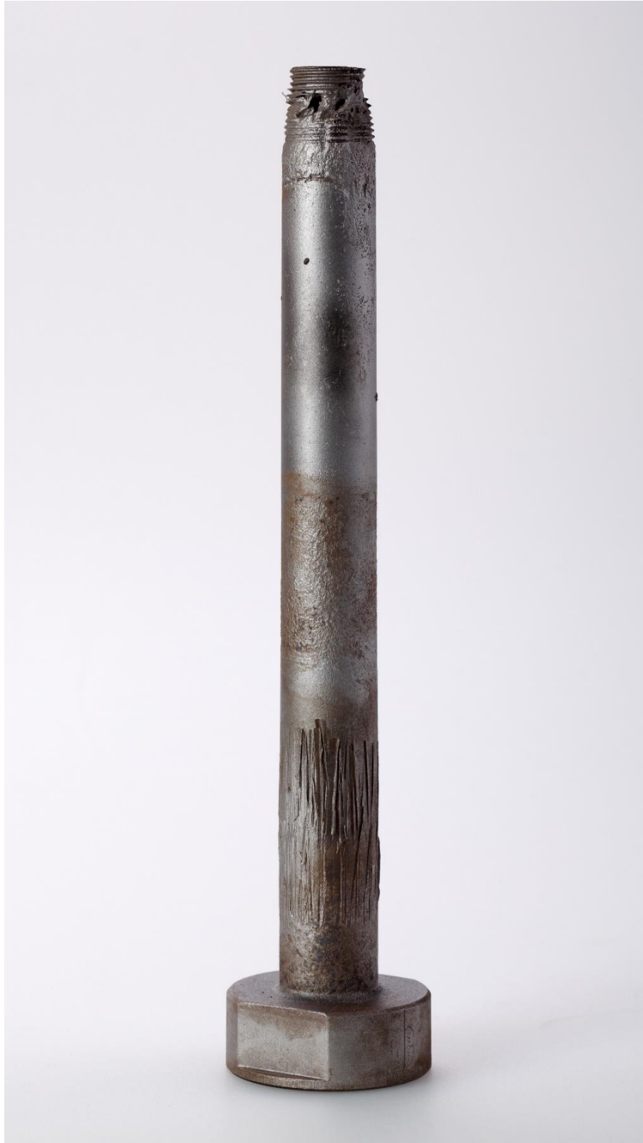
Corrosion and erosion at a steam nozzle © CEphoto, Uwe Aranas
