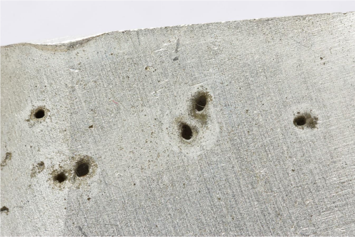
Damage mode: Pitting corrosion in a piece of aluminium. The holes caused by pitting which can be observed in this image are about 1 mm in diameter © CEphoto, Carlos Delgado
