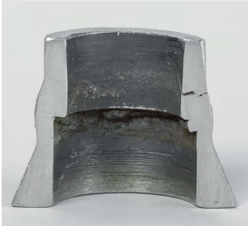
Damage Mechanism: Stress corrosion cracking of a quench pipe. Material: 1.4541 © CEphoto, Uwe Aranas
