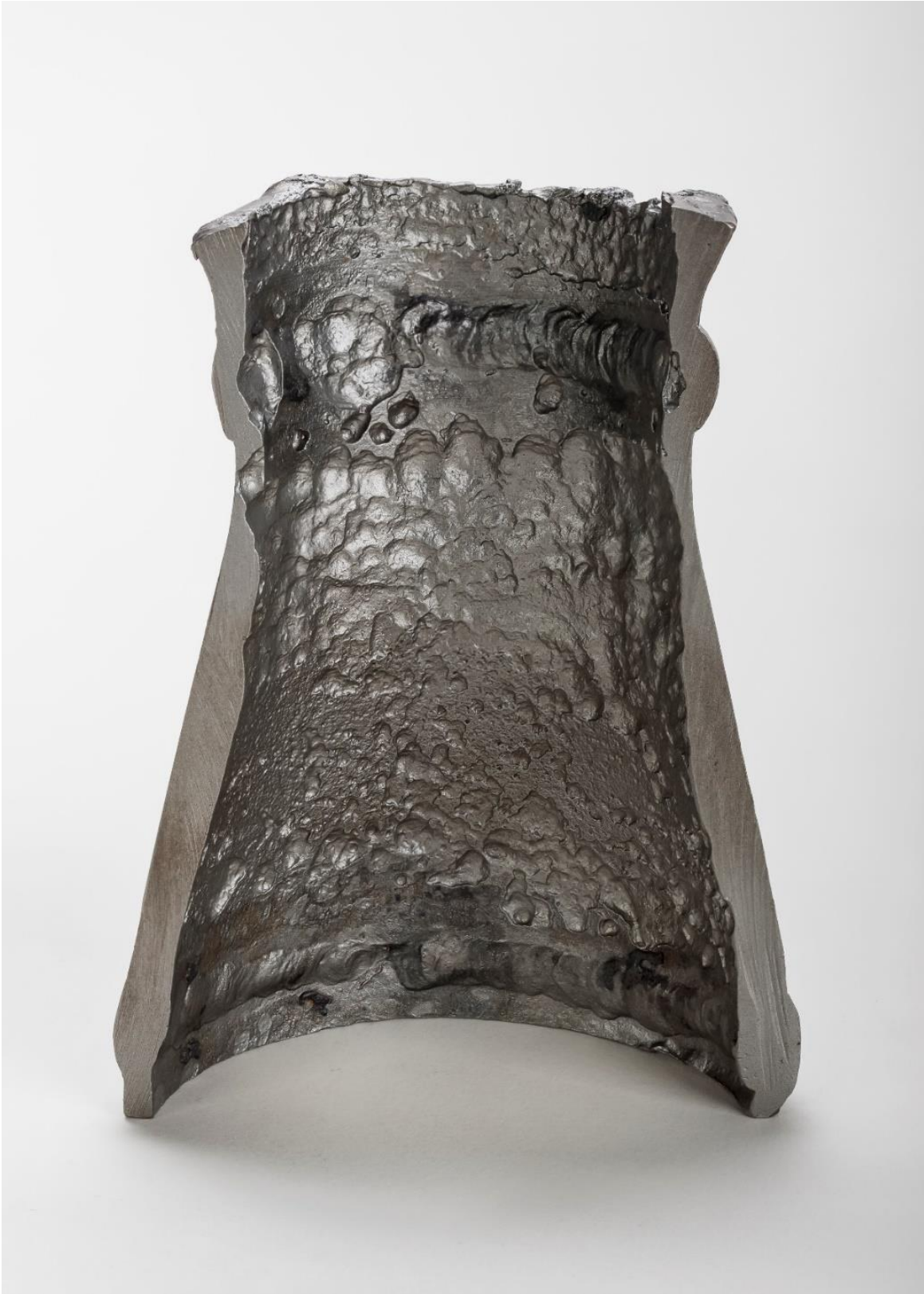
Damage Mechanism: Sulfolane corrosion in a pipe reducer. Damage mode: general thinning. © CEphoto, Uwe Aranas
