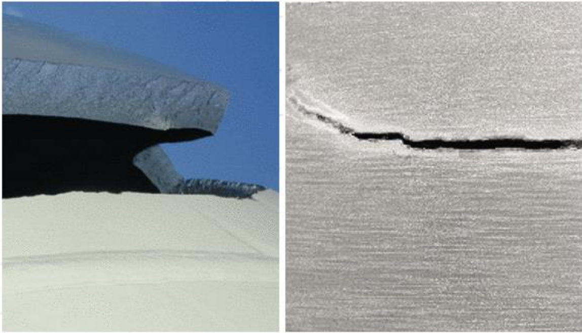
Damage mechanism: Brittle Fracture. Damage mode: Failure mode: Rupture. CC Caroline Phoenix
