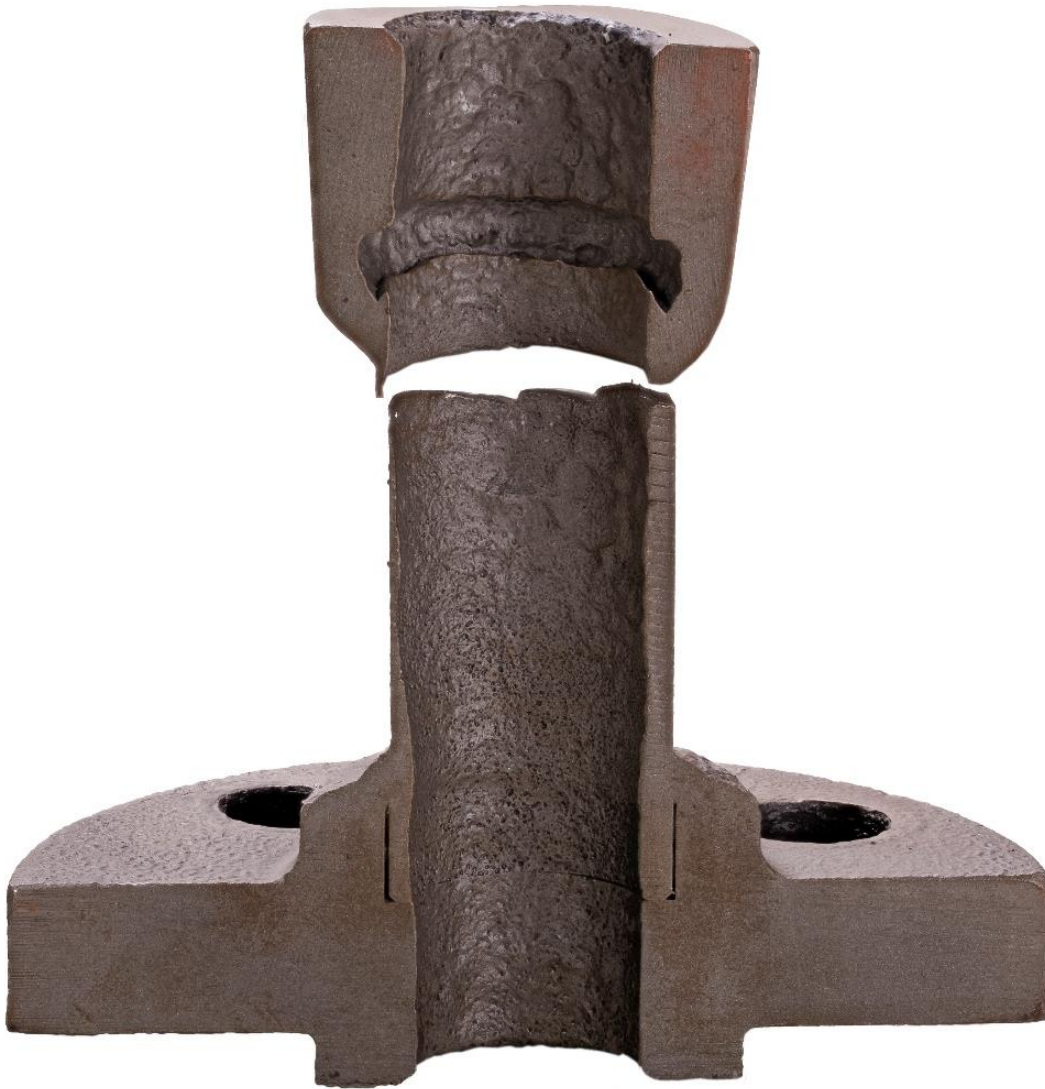
Damage mechanism: High-temperature sulfur corrosion of a 12 CrMo 19.5 pipe stub (used for insertion of a pressure indicator) © CEphoto, Uwe Aranas
